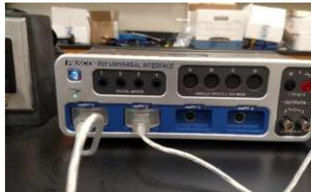
Connections for two new motion sensors.
